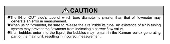
The tube can be mounted in horizontal, vertical and diagonal. However, in any case, the tubing system must be filled with the liquid at all times.
