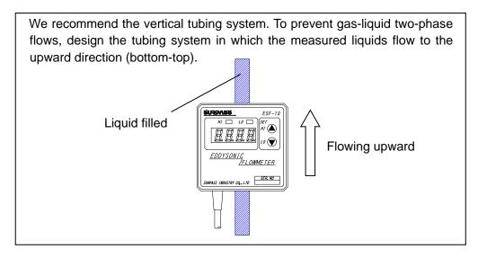
Design straight-tube parts on both sides of flowmeter. The straight-tube length of IN side must be at least 7 times longer than the bore diameter, and that of OUT side must be at least 5 times longer than the bore diameter.
