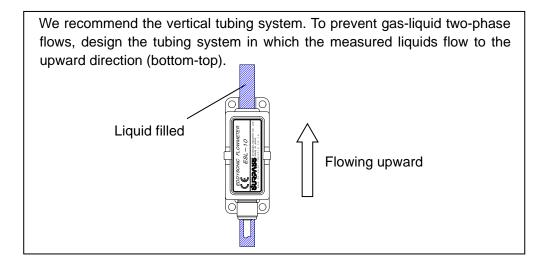
Design straight-tube parts on both sides of flowmeter. The straight-tube length of IN side must be at least 7 times longer than the bore diameter, and that of OUT side must be at least 5 times longer than the bore diameter.
