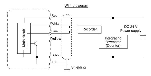
XBlack, Blue and F.G leads are connected each other within the circuit.
