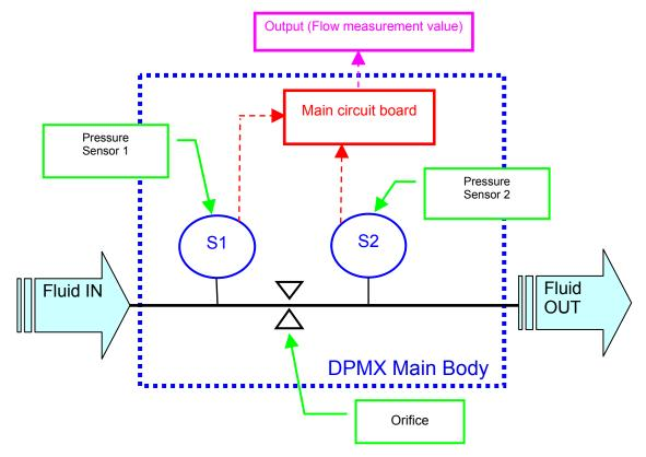
When liquid is fed into the main body, pressure differences occur before and after the orifice.
