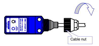
(2) Grasp the cable bush and pull out the cable.
