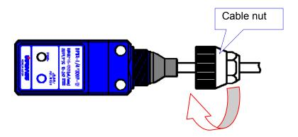
(3) Securely tighten it until there is no space left between the main body and the cable nut.
