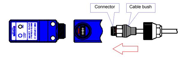
(2) Turn and loosen the cable nut in the illustrated direction and tighten it on the main body.
