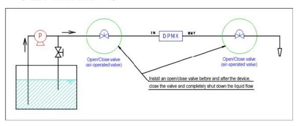
\* When flow rate zero adjustment is performed under piping conditions other than those listed above, proper zero adjustments cannot be performed.
