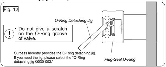
Attach a new O-Ring to the O-Ring groove of valve and adjust it until it can be fitted to the groove.
