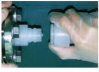
Insert the socket into the plug by pulling the socket sleeve until the head of socket reaches the plug.
